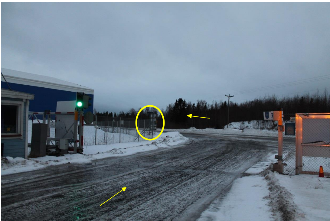
Pic 2/pos A1. Turning after gate toward Satamatie (road 7771). Marked part of fence and sign need to be removed if transports are longer than 45m. Yellow arrow points driving direction.
