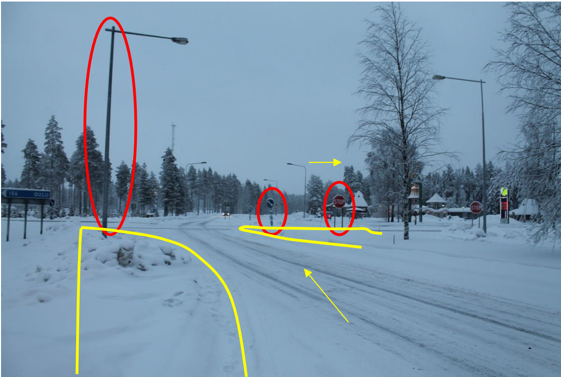
Pic 37/pos 19. Turning from road 27 toward road 4. Marked lamp post and signs need to be removed. Marked areas need to be filled. Yellow arrow points driving direction.
